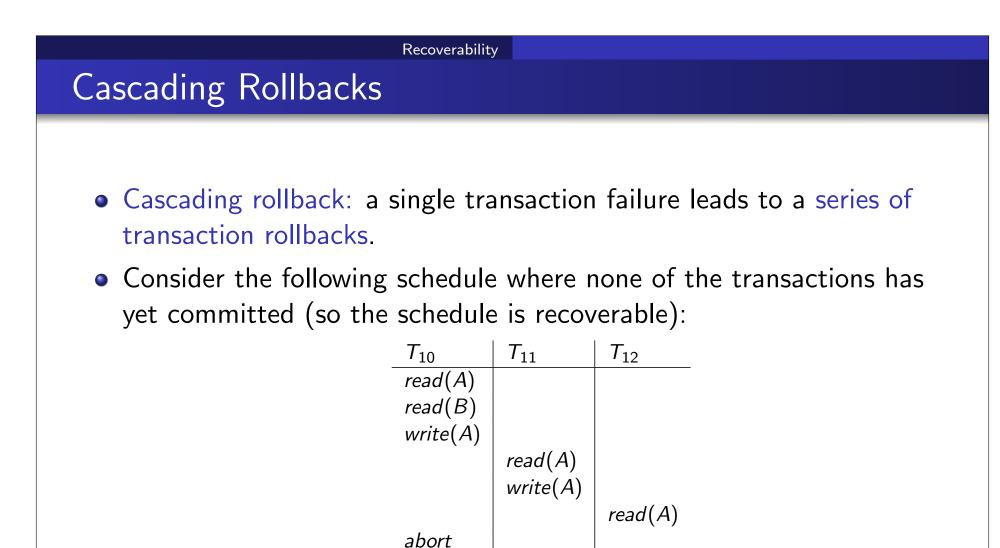
If  $T_{10}$  fails,  $T_{11}$  and  $T_{12}$  must also be rolled back.
