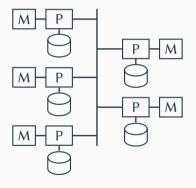
$P \dots processor, M \dots memory, \Theta \dots disks.$
