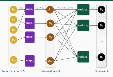
Each task (map/reduce) runs on a node, i.e., a node can be mapper *and* reducer.
