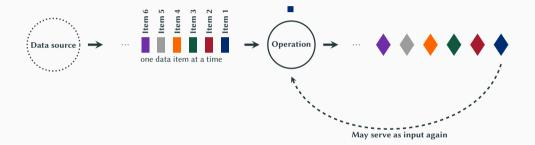
**Stateless Processing:** The **current operation processes** the **input data independently**, i.e., without considering preceding executions. The independence of the state makes it easier to scale.
