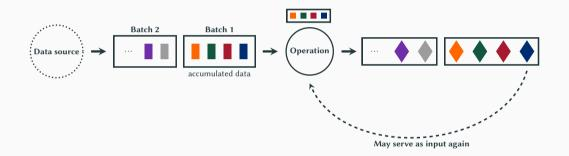
We do not wait for the data to accumulate but **process each single data item continuously** (at arrival). This allows a real-time response and typically involves simple transformations.
